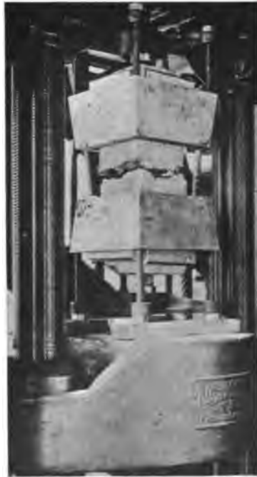
FIG. 104.—Tensile Test of Concrete.
